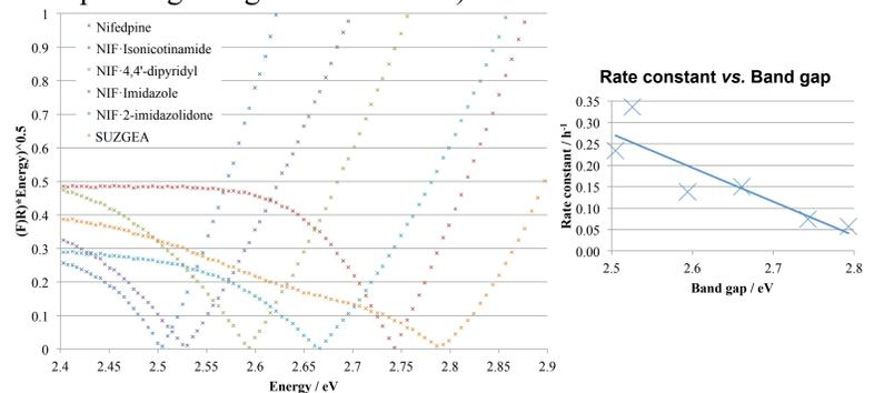
Fig. 6 - a) Tauc plot for NIF and its cocrystals. The extrapolation of the straight line to the x-axis corresponds to the band gap. b) The rate constant for degradation plotted against the band gap for NIF and its cocrystals indicating that the larger the band gap, the slower the rate of degradation.
