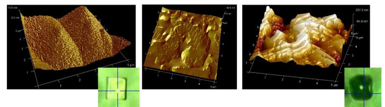
Fig. 7 - AFM height images: a) NIF pre-degradation showing molecular steps. b) NIF during degradation, (flat parts are amorphous). c) NIF post-degradation, surface is highly disordered indicating multiple nucleation points. (inset - optical microscope images of NIF pre- and post-irradiation)
