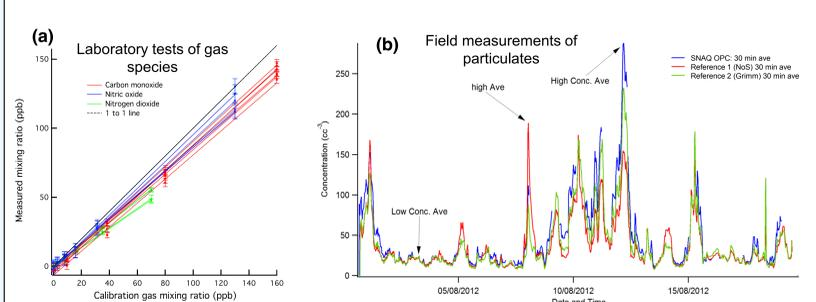
Figure 3: Laboratory calibration<sup>1</sup> (a) of CO, NO, NO<sub>2</sub> sensors against gas mixing ratios and time series showing field measurement comparison between 30 minute average OPC measurements and two reference particle instruments.
