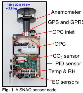
Fig. 1: A SNAQ sensor node
