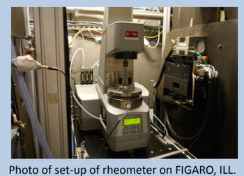
Photo of set-up of rheometer on FIGARO, ILL.
