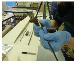
Carefully painting the polymer onto a wood sample
