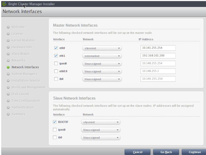
Figure 2.8: Network Interface Configuration
