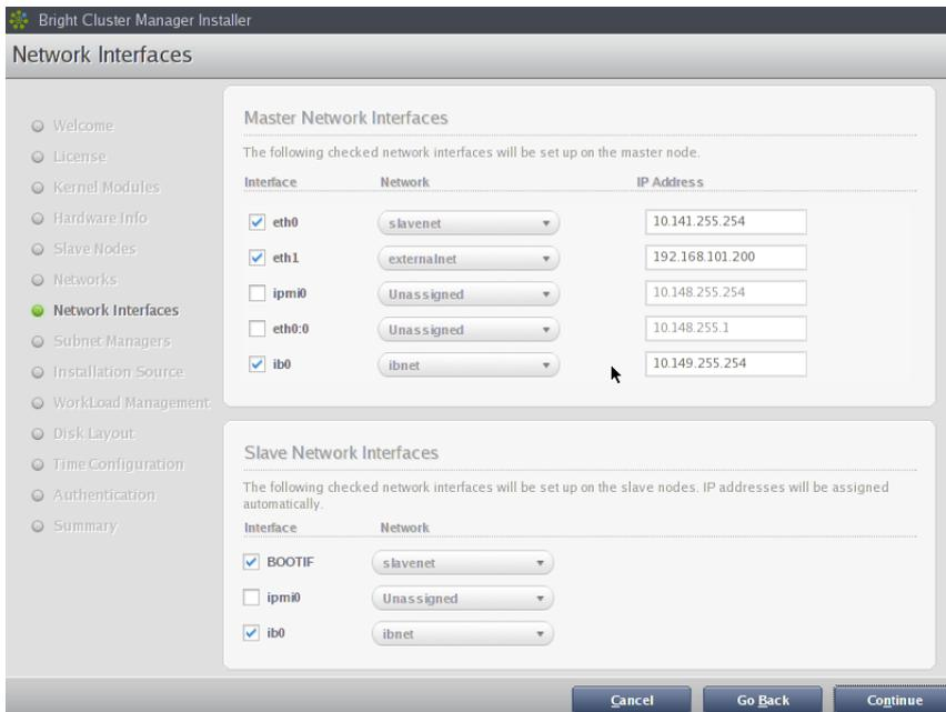
Figure 2.9: Network Interface Configuration - Infiniband interface enabled
