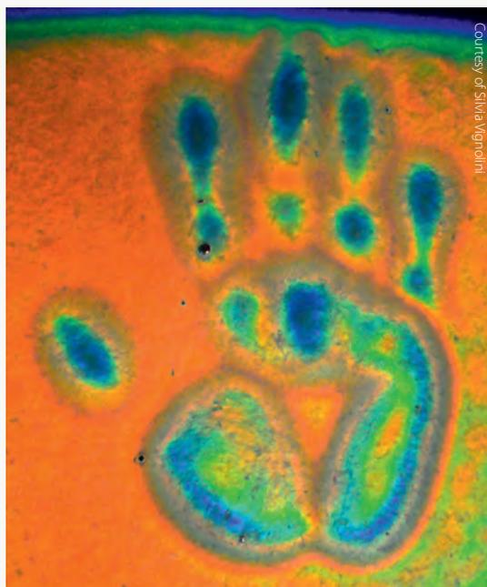
**The image shows a hand pressing onto the HPC strain sensor. As the strain pattern of the hand is applied, the pressed region of the sensor shows a vivid blue colour. The different colours produced correspond to varying amounts of pressure. The colour change is reversible when the pressure is removed.**
